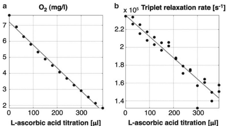
**Fig. 39.3** Observation of TMR adhering to a glass cover slide in a flow cell. Titration of 25.5 mM L-ascorbic acid removes the oxygen in controlled discrete steps. (a) Dissolved oxygen as measured by a commercial probe. (b) Triplet state relaxation rate  $k_T = 1/\tau_T$ . Reprinted from [1]
