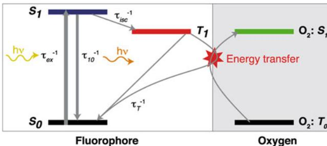
**Fig. 39.1** Jablonski diagram of a fluorescent molecule illustrating the three basic energy states of the molecule. Molecular oxygen exhibits a triplet configuration in its ground state which allows it to accept energy transfers from the triplet state of the fluorescent molecule. Reprint from [1]
