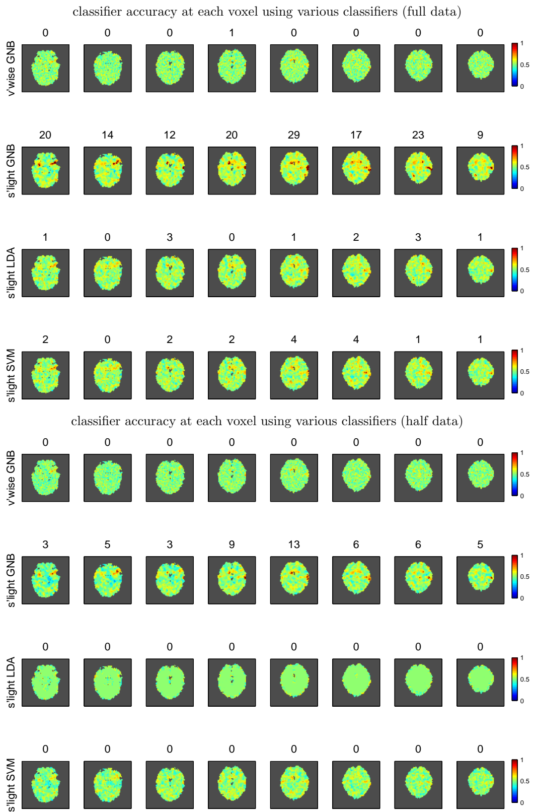
Figure 5: Comparison of accuracy maps obtained with 6-fold cross-validation (top) and 2-fold cross-validation (bottom); the former have \frac{5}{6} of the data to train on, the latter only \frac{1}{2} . For both plots, each row contains eight slices from an accuracy map, inferior to superior, top of each slice is posterior. The classifiers used in each row are single voxel GNB and radius 1 neighbourhood GNB, LDA and linear SVM. On top of each slice is the number of voxels for which accuracy was deemed significant using FDR q = 0.01 , which are highlighted in dark red.
