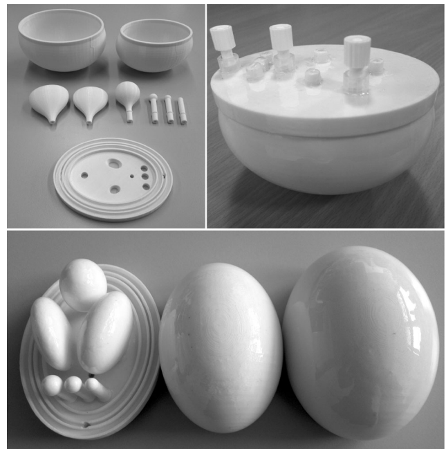
FIG. 2. Top left: Printed phantom components. Top right: Completed phantom. Bottom: Partially assembled phantom following application of epoxy coating.
