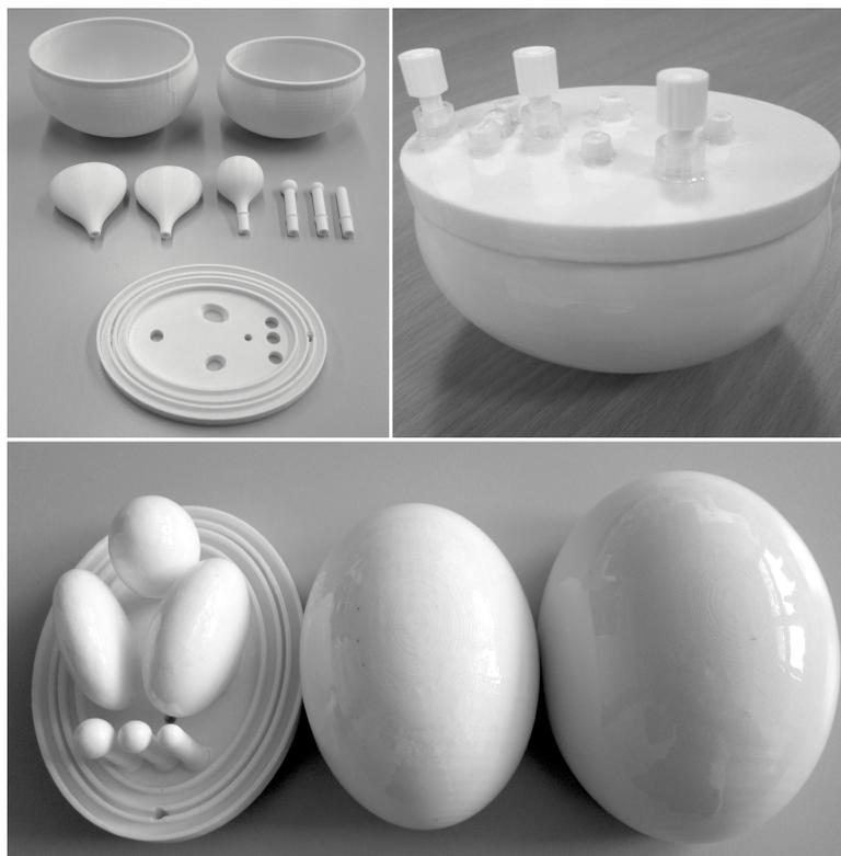
Figure 5.3: (Top/Left) The printed phantom components. (Top/Right) The completed phantom. (Bottom) The partially-assembled phantom following application of the epoxy coating.
