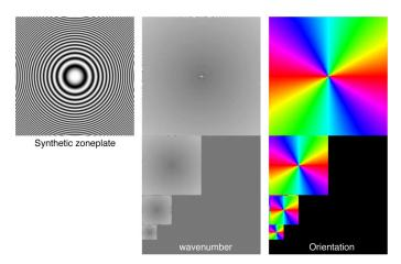
Fig. 7. Example of wavelet-domain monogenic image analysis. Left: Input image (synthetic zoneplate); center: wavelet-domain wavenumber estimation with calibrated frequency scale. Right: Tensor-based orientation (Hue channel).
