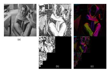
Fig. 9. Example of wavelet-domain coherence analysis. (a)  $512 \times 512$  Barbara; (b) wavelet-domain coherency map; (c) composite HSB display of results (Hue: orientation, Saturation: coherency, Brightness: amplitude).
